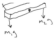
The suspended masses try to rotate the bar The turning effect or moment of the force is determined by the force and the perpendicular distance of its line of action from the point.
