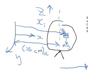
IF the object is balanced, the centre of mass is directly above the support Consider an element of the object at distance  $x_i$  from the z axis. The centre of mass is a distance  $(\underline{x}_cm)_x$ from the z axis
