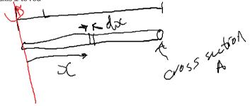
Slice the rod into short sections of length dx. Volume of element dV=Adx The rod is uniform  $=>\rho=$ constant
