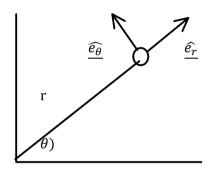
These are "natural directions in polar coordinates Why didn't we work in these directions from the start? The radial and tangential directions depend on position \*here be dragons\*
