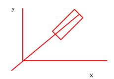
If the axel makes an angle  $\theta$  to the x-axis  $\bar{L} = \begin{pmatrix} Lcos\theta \\ Lsin\theta \\ o \end{pmatrix}$
