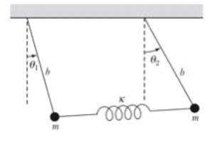
$\begin{aligned} x_+(t) &= A_+ \sin(\Omega_+ t) \to \Omega_+ = \omega_p \Rightarrow \text{slow mode} \\ x_-(t) &= A_- \sin(\Omega_- t) \to \Omega_- = \sqrt{\omega_p^2 + 2\omega_s^2} \Rightarrow \text{fast mode} \\ \text{Most general solutions is a linear combination of } x_+ \& x_- \\ A_+ \sin(\Omega_+ t) + A_- \sin(\Omega_- t) \end{aligned}$
