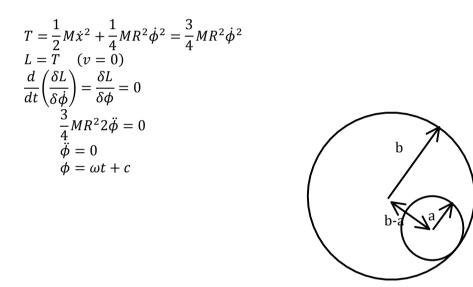
Small cylinder rolling without slipping inside bigger hollow cylinder
