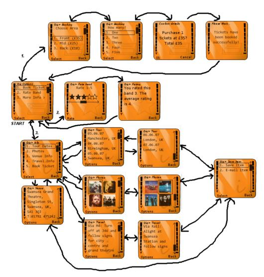
The above diagram demonstrates the typical usage pattern of the system.
